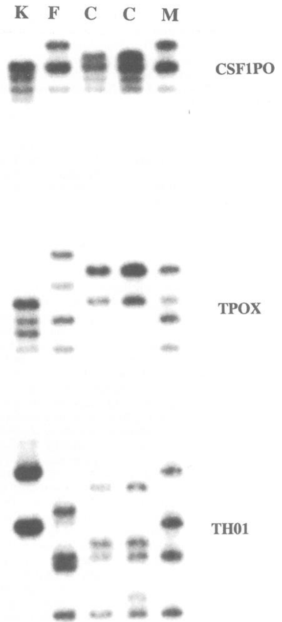
FIG. 3—SSCP of loci CSF1P0, TPOX, and TH01. The products of multiplex PCR were mixed with denaturing loading buffer, heated at 94°C for 2 min and chilled in ice water. Electrophoresis was done in 6% non-denaturing acrylamide and the temperature of the plates was below 40°C. Bands can be identified in the loci CSF1P0 (top), TPOX (middle), and TH01 (bottom). K refers to K562 cells, F to alleged father, C to children, and M to the mother's DNA.
